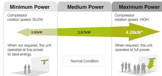
Graph shows the 1.5HP Inverter model's wide power output range during cooling.
